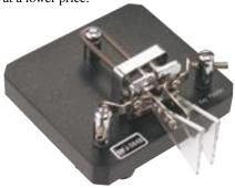
As with the Bencher, the adjustment of spring tension is possible, but only over a limited range through the adjustment of the pivot stop screws and then readjustment of the contact spacing to compensate. Use of a standard hex wrench is required for adjustment of the pivot stop screws. The contact spacing is also adjustable via a hex wrench. If the Phillips locking screws are loosened, however, the contact spacing can be adjusted by hand and then locked into position. No tools are supplied.
