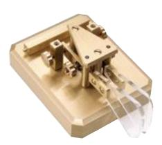
simple, but it is elegantly executed. The Dirigent employs needle and seat bearings rather than the ball bearings more commonly found in high quality paddles. The seat is so precisely machined that the bearings are known to last for many years without any adjustment. The levers are brass, so more mass is moved with each stroke than is needed for lighter levers.
